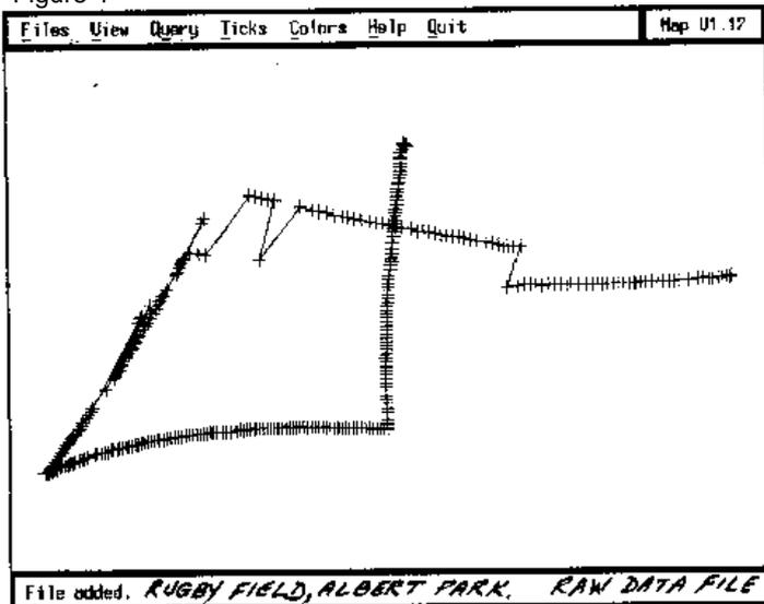
ure 1, clearly demonstrates the possible degradation of positional accuracies which pertain to all GPS receivers. Differential correction through GEO-PC software took a matter of minutes, the results of which are shown in Figure 2
