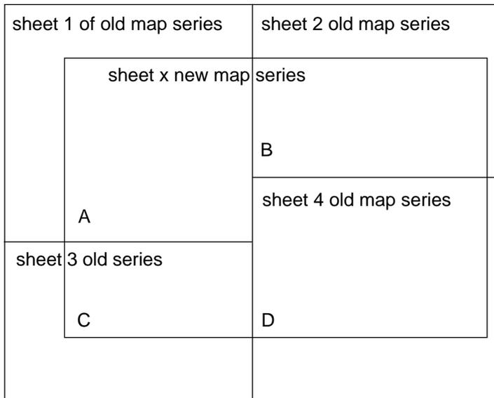
Figure 2. Overlap of map sheets from the old and from the new series. The GISMO program of ERDAS cuts out of the sheets 1, 2, 3 and 4 the parts A, B, C and D which cover the map sheet x of the new map series.
